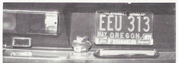
Mounting by Steve Howell. Detach bumper, lower it, drill mounting holes so that bumper will conceal them when in place.
