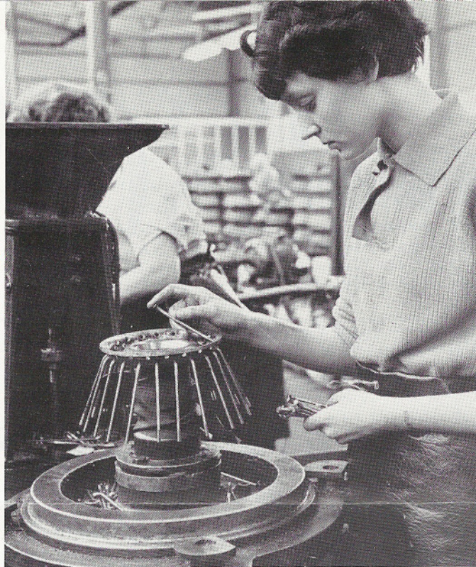
The spokes are assembled into the hub by hand, then the rim is added and the whole works tightened together.
