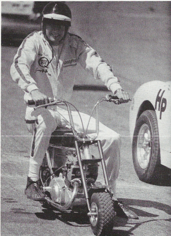
Brian Fuerstenau leads in the great mini-bike competition. Powered by a 150 cc Honda twin, his new creation looks potent enough to out-run the HP Sprite.
