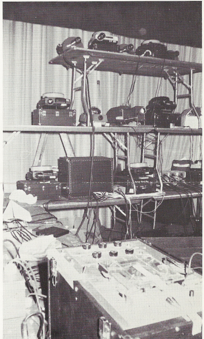
25-circuit control board in foreground runs myriad lights, projectors, tapes, etc. Need top electrician or spaghetti chef!
