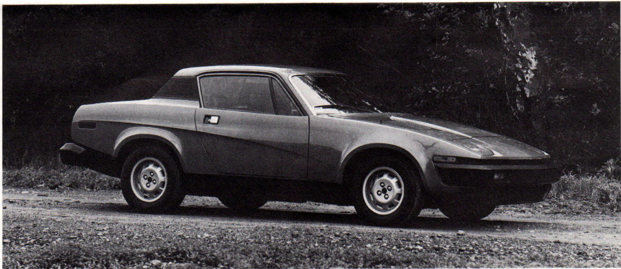
TR7's modernistic wedge shape has become familiar on American roads. Unchanged in exterior styling for 1978, it incorporates air dam, restyled wheels and lower rear end from the revisions of last year.
