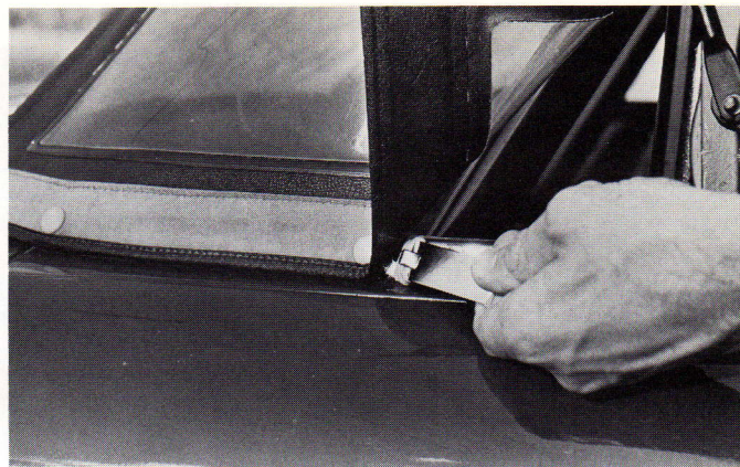
Here is the simple instrument invented by Wilhelm Herhaus for reluctant soft-top press buttons. They can be mastered by a can opener, insulated with rubber bands to prevent paint damage.
