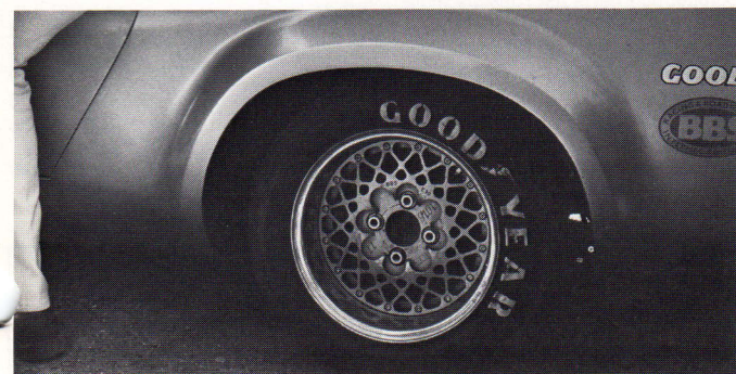
The West Coast TR-7 uses a special type 3-piece alloy wheel, which is adjustable for various rim widths.
