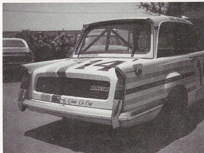
Back view shows the roll cage inside, fender flares, cap for safety fuel cell and central exhaust. Car has 2-litre, 3-Weber Triumph six, suspension similar to GT-6 Mk 3.
