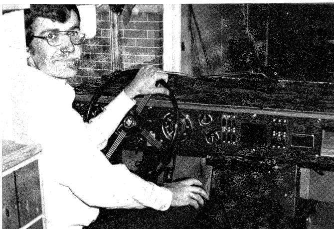
The nicely fitted dashboard of unique construction. Wiring and components are mounted in a box with removable lid.
