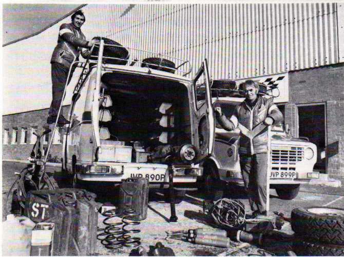
Triumph rally servicing in Europe is undertaken by a pair of Leyland Sherpa light commercial vehicles of a type not marketed in the U.S. Chosen for their big load carrying capacity, good interior access and economy, these "barges" (rally slang for service vehicles) are mobile workshops and spares departments. Equipment includes welding and cutting gear, trolley jacks, air bottles, spare parts racks, and roof racks for a variety of rally tires.
