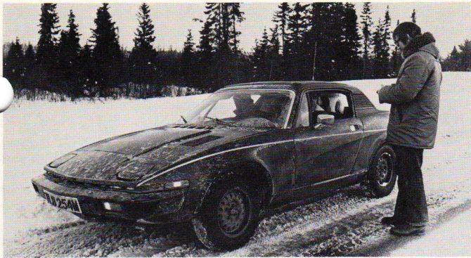
Partially disguised with false trim and wheels, TR7 underwent weeks of below zero, cold weather tests in Northern Canada.
