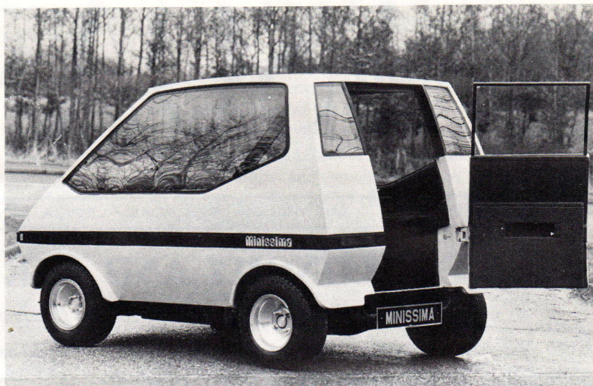
TOWN CAR FOR THE ENERGY CRISIS: British Leyland exhibited this pint-size, 40 mpg 'idea car' at the Chicago auto show which concluded March 3. Only 7½ ft. long, it can carry four passengers and make a U-turn in 20 ft. It's not a Triumph but uses engine, transmission and suspension from the famous Mini. You can see it again at the New York Show, April 6/14.
