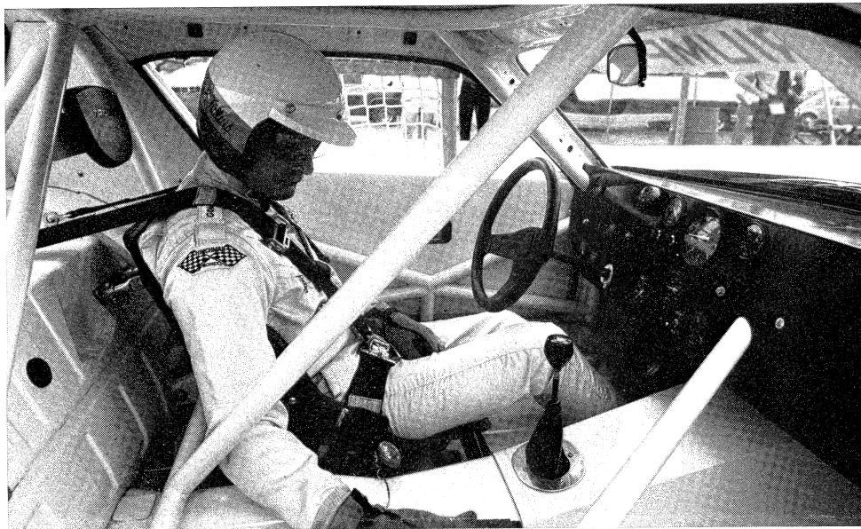
A cockpit view of Bob Tullius, Group 44's team leader (above and left) at Daytona where he put up such high speeds. Strapped in his 6-point harness, he is checking the console of switches on the 'passenger' side—for ignition, starter, fuel pump, differential oil cooler, wipers, etc.
