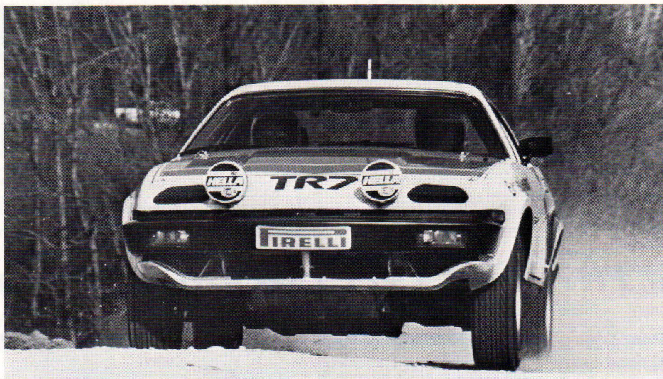
The rally TR7 at speed. Some sections are covered at over 100mph. Note the oil sump shield and high ground clearance.
