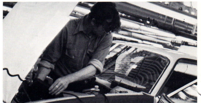
After the curved windshield is installed, it is bonded into place by fusing the mastix electrically. Here the line man switches on the current for a limited time.
