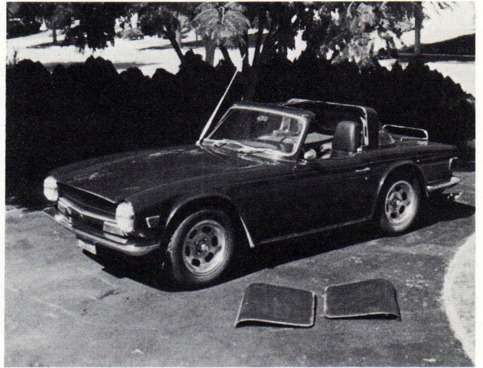
TR6 (135,000 miles) owner Steve Latshaw of Canoga Park, California, has built a fiberglass top with removable roof sections, which can be stowed behind the seats.
