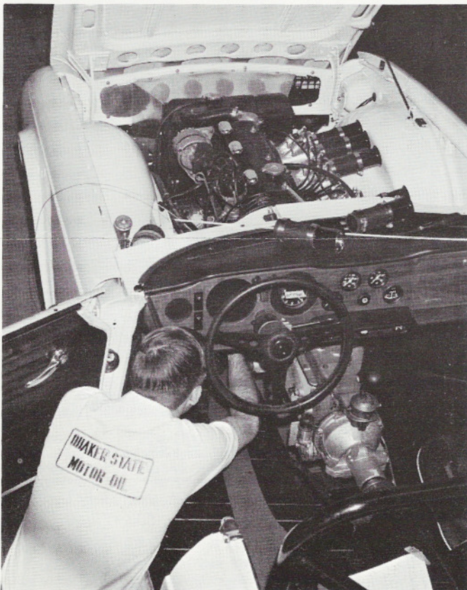
Brian Fuerstenau digs under the TR-6 dash, adjusting the throttle linkage. Visible items: Fuel injection system with six individual velocity stacks, special valve cover vents, "hot plugs" warning note on tach.
