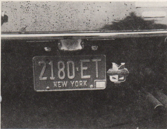
John Morano's rear mount on GT. Many hardware store metal strips would work.
