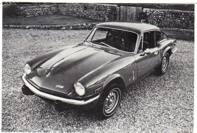
Power assisted front disc brakes, wider rear track and tinted glass all-around are the key features of the 1973 Triumph GT-6 fastback coupe. The six cylinder sports car also has interior modifications including improved seats and instrument graphics.
