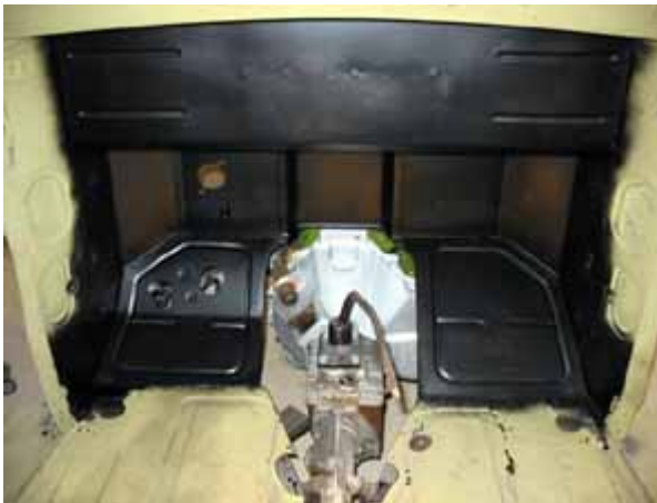
New firewall, foot wells and front floor boards from passenger compartment.
