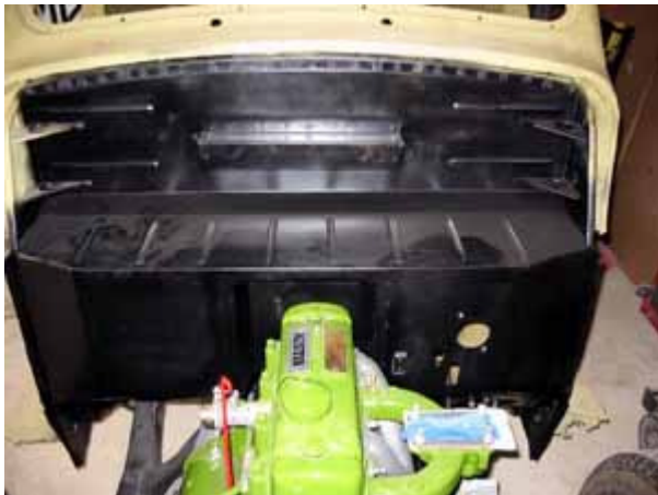
New firewall sheet metal from inside engine compartment
