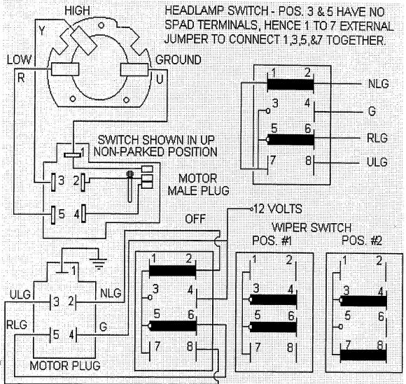
Take notice that the color coding for the wiring harness and the motor are not the same. The parking switch is shown in its up or non parked position (plunger not held down by the parking cam).
