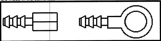
This is a great "on the side of the road" quick fix and you only have to carry a length of rubber fuel line hose and a couple of clamps. Insure that the spare hose is designed specifically for use with petrol.
