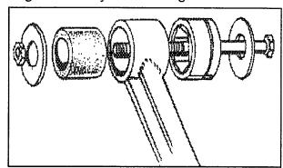
completely pressed in its mounting, disassemble the rig, and check for its proper position within the mounting hole. You will be surprised at just how easy the bushing will press in place. Of course, if the part with the mounting hole has been removed from the car, I prefer to use a socket and my bench vise.
