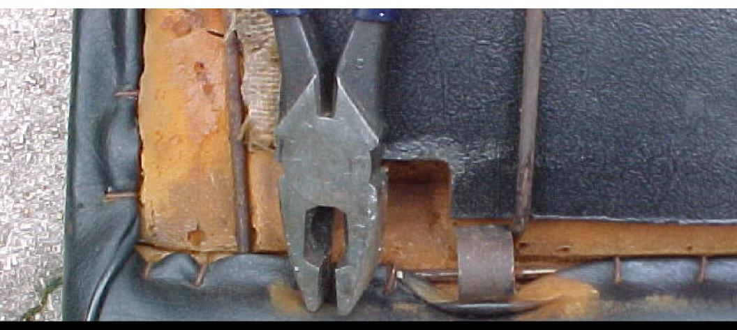
WITH THE BOTTOM FREE FROM THE FRAME, USE HEAVY PLIERS TO WREST THE HOGRINGS FROM THE SEAT BOTTOM FRAME. NOTE HOW VINYL IS BUNCHED UP AND THE HOGRINGS PIERCE THE VINYL TO HOLD VINYL TO FRAME.
