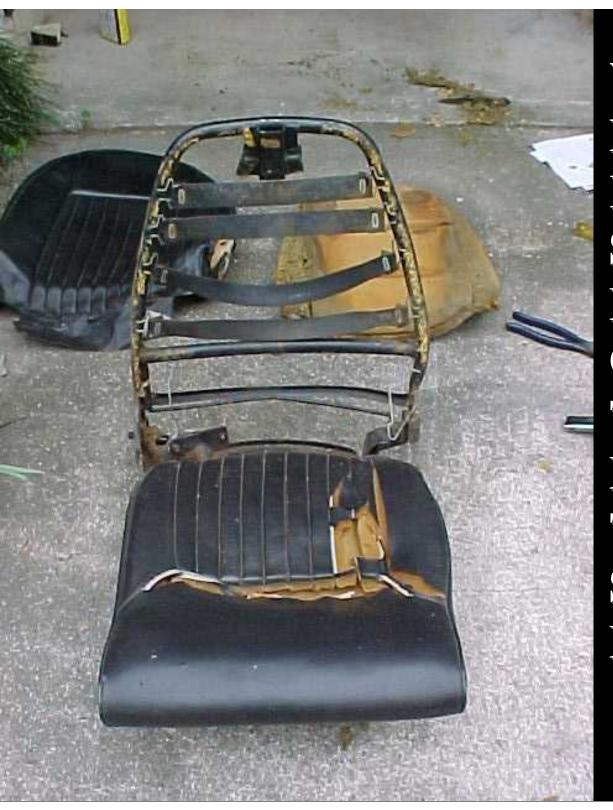
WE'RE DEFINITEDAY REPLACING THE SEAT BACK FOAMS! PULL 'EM OFF GENTLY -THEY ARE MERELY GLUED TO THE **SEATBACK** FRAME.
