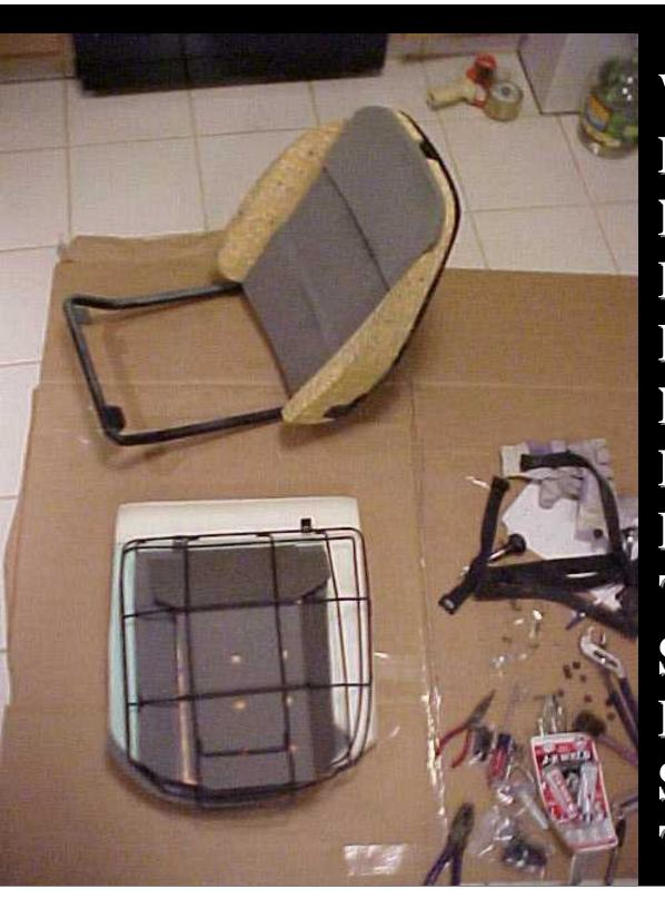
WITH WEBBING DONE, GLUE THE NEW SEAT BACK FOAM TO THE FRAME. NOTE NICE, NEW BLACK PAINT. ALSO, TRY RITTING TOGETHER THE **SEAT BOTTOM FOAM AND SUPPORT BOARD** TO LOWER FRAME
