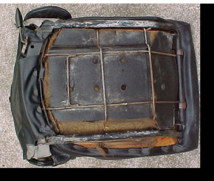
NOTE PLACEMENT OF CLIPS, HOGRINGS BEFORE DISASSEMBLY. REFER TO OTHER SEAT WHEN IN DOUBT.
