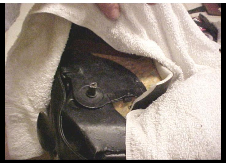
SPRAY ADHESIVE TO FINISH BOTTOM EDGE OF SIDE BOARDS AND EXCESS VINYL FLAPS. PULL THE BOARDS DOWN AND SEAT THE CLIPS INTO THE FRAME. CUT OUTER HOLE FOR RECLINER LEVER NOW...
