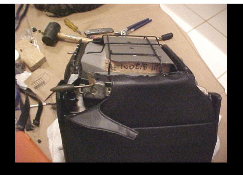
WE ARE ALMOST FINISHED! INSTALL HOLD-DOWN LEVER AND CLIP DOWN THE SEAT BACK COVER TO LOWER FRAME.
