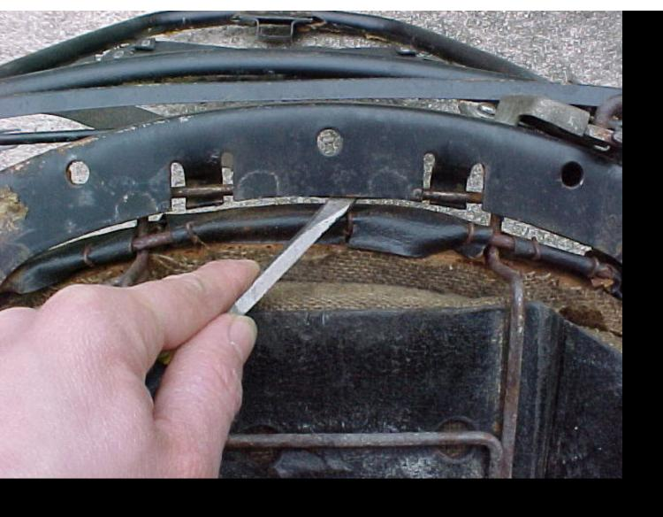
PRY THE SEAT BOTTOM FRAME FROM THE CAGE WITH A SCREWDRIVER. IT MAY BEND THE SHAPE - BEND BACK WITH PLIERS LATER.
