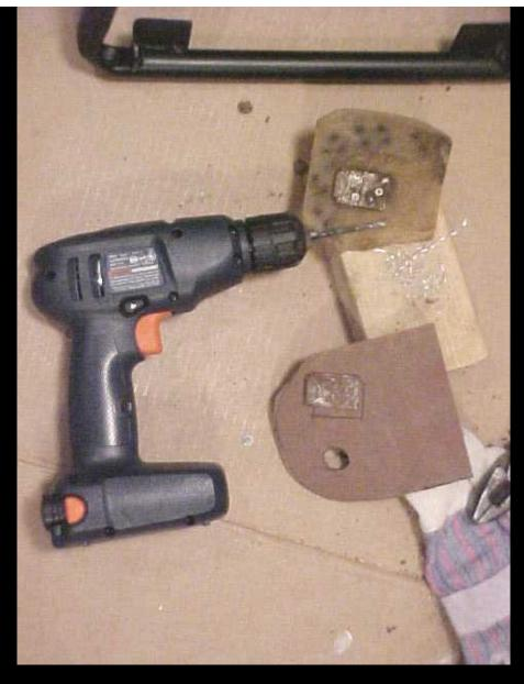
DRILL OUT RIVETS SO WE CAN RE-USE THE ORIGINAL CLIPS. IT'S IMPT. TO MAKE THE NEW SEATS FIT WELL AND NOT SAG...
