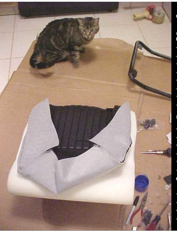
TOP VIEW OF **SEAT BOTTOM** FRONT. HOG RINGS ALREADY INSTALLED ON REAR OF VINYL COVER TO THE **BOTTOM SEAT** FRAME. MR. KITTY'S LOOKING TO GET HURT IF HIB SITS HERE NOW!
