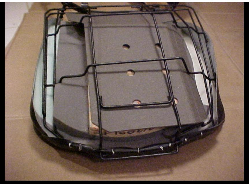
INSTALL THE HOGRINGS! BEGIN BY PULLING THE VINYL OVER THE FOAM AND INSTALL RINGS AT REAR OF SEAT FIRST...
