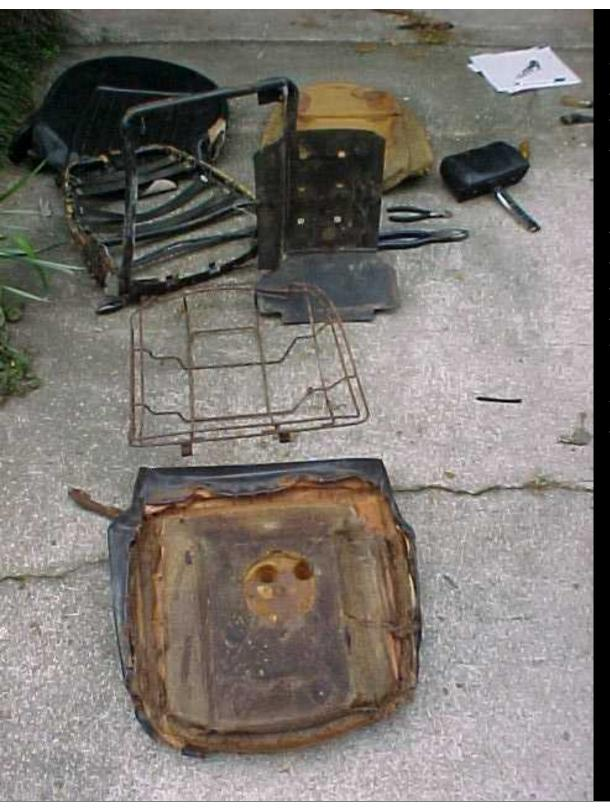
NOW, THE FOAM/VINYL IS SEPARATED FROM THE SEAT BOTTOM FRAME. WE ARE USING NEW FOAMS, SO THERE'S NO NEED TO SEPARATE THE FOAM FROM THE VINYL...
